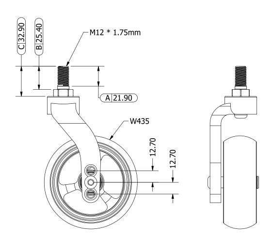
\*1: Dimension "A", "B", "C" & Thread size can be customized. \*2: All dimension in "mm".
